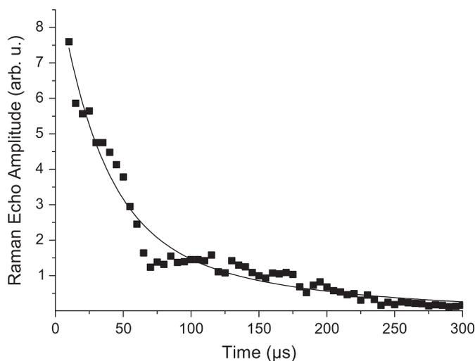
**Fig. 3.** Raman echo amplitude for the  $\pm 1/2g \rightarrow \pm 3/2g$  transition as a function of the pulse separation in a 3% Pr:La<sub>2</sub>(WO<sub>4</sub>)<sub>3</sub> sample (squares) and fit by a two exponential function (solid line).
