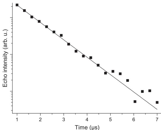
**Fig. 4.** Photon echo decay (<sup>3</sup>H<sub>4</sub>(0) → <sup>1</sup>D<sub>2</sub>(0) transition) as a function of the pulse separation in a 3% Pr:La<sub>2</sub>(WO<sub>4</sub>)<sub>3</sub> sample.
