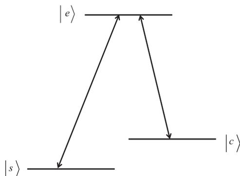
Fig. 1. A three level  $\Lambda$  system.  $s$  signal ground state level,  $c$  control ground state level,  $e$  excited level.
