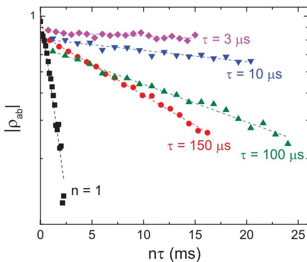
FIG. 6. (Color online) Measurement of  $T_2$  through CPMG sequences with different  $\tau$  values. For data sets labeled  $\tau = 150, 100, 10$ , and  $3 \mu\text{s}$ ,  $\tau$  is kept fixed and  $n$  is increased. The data set labeled  $n = 1$  is a standard spin-echo experiment ( $n$  is fixed and  $\tau$  is increased). The dashed lines result from least-squares fits.
