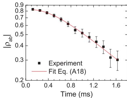
FIG. 4. (Color online) Spin-echo experiment.  $|\rho_{ab}|$  is obtained from the quantity  $\ln(I_f/I_{ref})/\ln(I_i/I_{ref})$ , where  $I_i$  and  $I_f$  are the transmitted probe intensities before and after the rf sequence, respectively, and  $I_{ref}$  is a reference intensity for a known population difference (typically 0). The fit returns the parameters  $\sigma_{\Delta}/(2\pi) = (2.3 \pm 0.2)$  kHz and  $\tau_c = (172 \pm 30)$   $\mu$ s.
