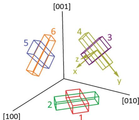
FIG. 1. (Color online) Orientations of the six orientationally distinct sites of the  $Y^{3+}$  ion in the YAG crystal lattice.<sup>36</sup> Each parallelepiped represents the local  $D_2$  symmetry for one of the sites. The  $\hat{x}$ ,  $\hat{y}$ ,  $\hat{z}$  axis are the local axis for site 4.
