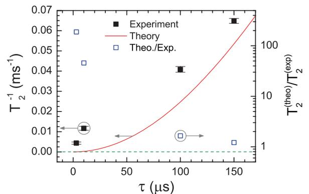
FIG. 7. (Color online) CPMG-extended  $T_2$  as a function of  $\tau$ . The experimental values (solid black symbols) result from the least-squares fit of the data of Fig. 6. The theoretical prediction (solid red line) represents Eq. (A16). The green dashed line indicates the lower bound  $(2T_1)^{-1}$  ( $T_1 \sim 1 \text{ min}$ ). The ratio between theoretical and experimental  $T_2$  values is also plotted (hollow blue symbols; these data refer to the right vertical axis).
