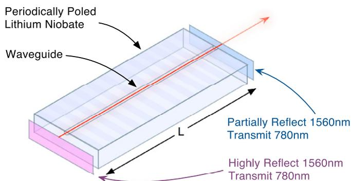
**Figure 1.** An integrated cavity-waveguide formed by reflection coating mirrors at the entrance and exit surfaces of a periodically poled nonlinear material.
