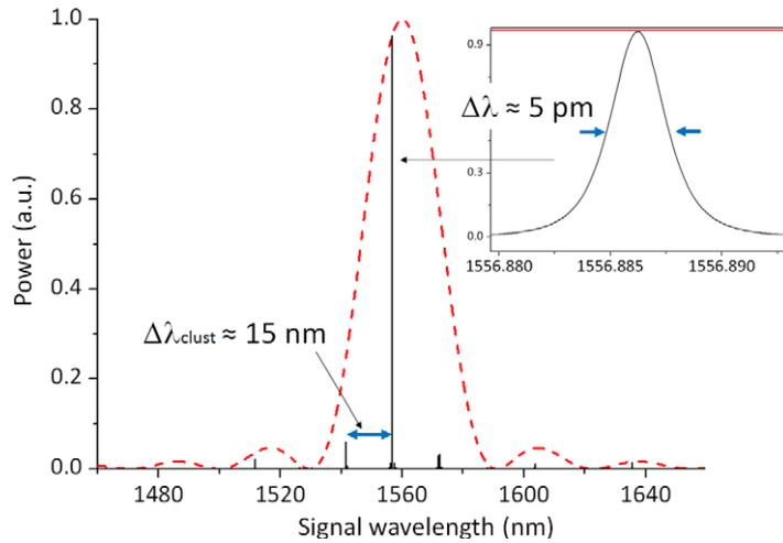
**Figure 6.** Frequency spectrum versus the signal wavelength, affected by the clustering effect, of an integrated cavity-waveguide whose parameters are indicated in the text. The red (dashed) line represents the phase-matching envelope. Right inset: zoom of the central single spectral mode.
