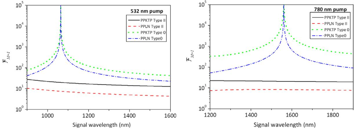
**Figure 5.** The finesse  $\mathcal{F}_{M=1}$ , corresponding to one mode in the clusters, for a 532 nm (left) and a 780 nm (right) pump, as a function of the signal wavelength. Type 0 (eee) and type II (eoe) interactions in PPKTP and PPLN are considered.
