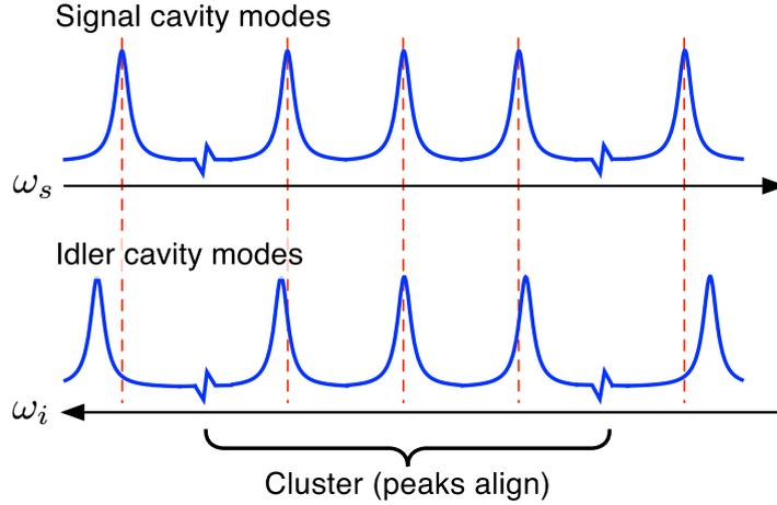
**Figure 3.** In a dispersive medium the optical length of a cavity varies with wavelength. SPDC occurs in such a cavity only when the double resonance condition is satisfied, i.e. when both signal and idler frequencies (satisfying  $\omega_p = \omega_s + \omega_i$ ) are resonant.
