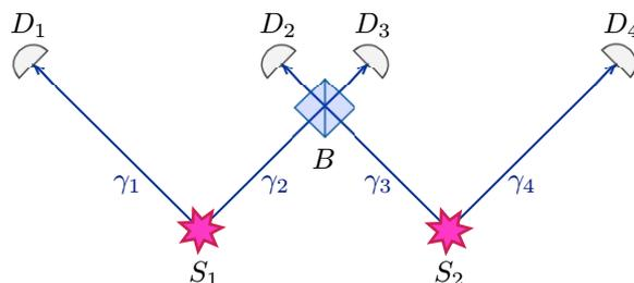
**Figure 7.** Photon interference scheme. The visibility of the Hong–Ou–Mandel interference of the photons  $\gamma_2$  and  $\gamma_3$ , which are heralded by the detectors  $D_1$  and  $D_4$ , respectively, is maximum when these two photons are in pure and indistinguishable states.
